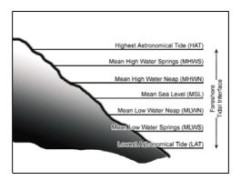
Figure 2: The Tidal Datums and the Tidal Interface
