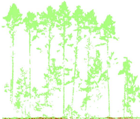
Figure 1 Result of ground classification with default values of parameters. Ground points are brown.
