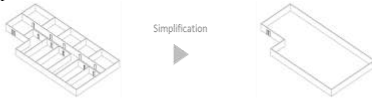
Figure 4. Simplifying BIM by using an algorithm excluding interior IFC objects.
