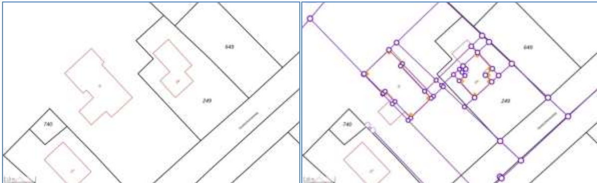
Figure 10: Cadastral map (legal boundaries in black, buildings in red) and on the right in overlay (purple) with the result of the adjusted survey measurements of the field sketch of Figure 2. Note that the map is oriented to the north while the field sketch of Figure 2 is not.
