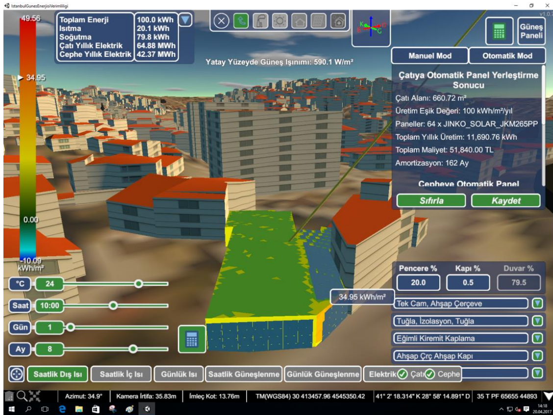
Figure 11. Solar estimation for the selected building rooftop and façade (potential solar panel)
