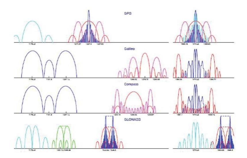
Signal spectra for GPS, Galileo, Compass, and GLONASS. From the left, new GPS satellites radiate at L5 (1176.45 MHz), L2 (1227.60 MHz), and L1 (1575.42 MHz)
