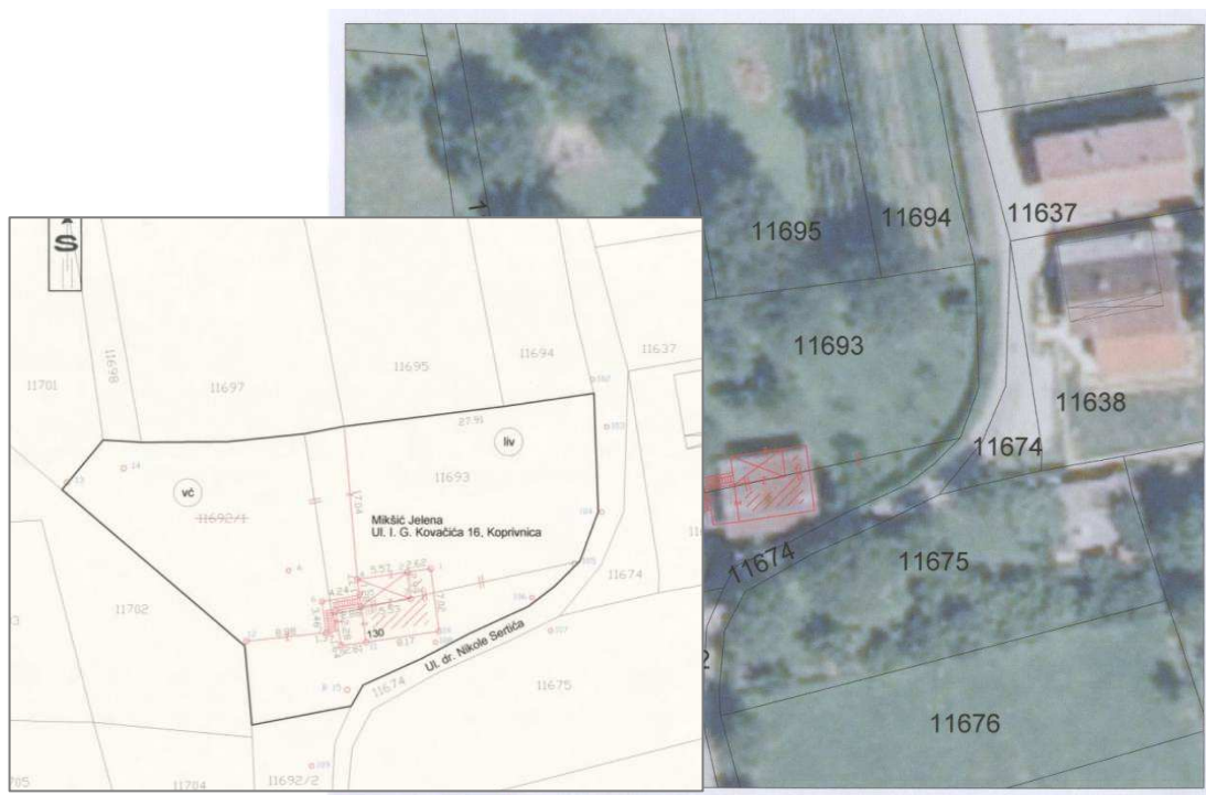
Figure 6 – Illustration of identical building in the cadastral map, survey sketch and DOP
