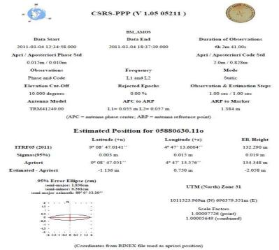
The existing orthometric height at the station is 108.669m while the derived above Geoid height using AUPOS – PPP was found to be 109.632m.
