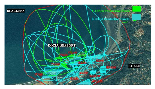
Figure 3 Influence areas of old and new production panels in Kozlu Seaport under active and residual subsidence influences.
