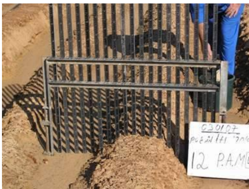
Fig. 2. Profile meters, a) common profile-meter, b) the proposed measuring-frame.
