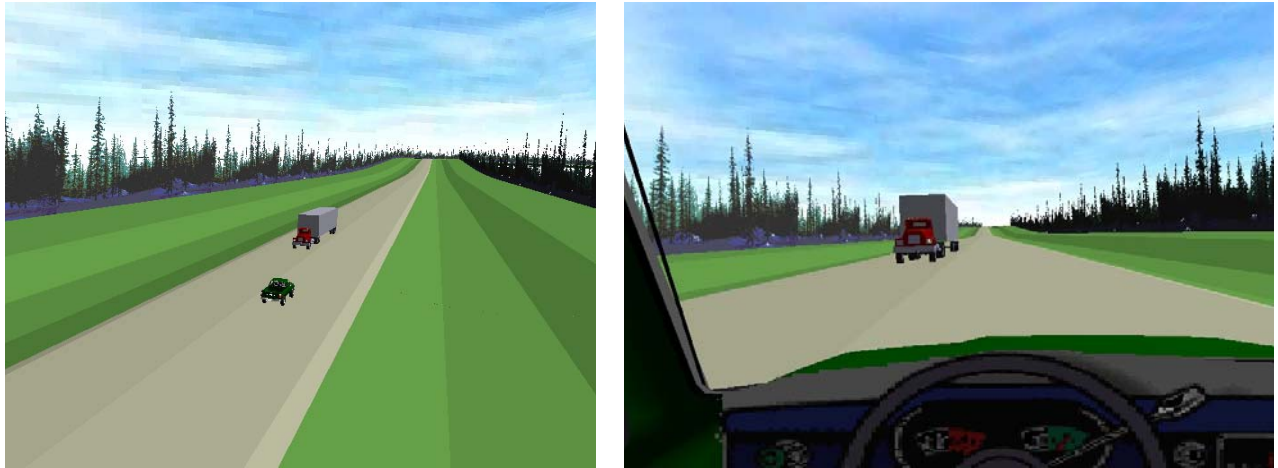
Figure 3: Bird's-eye and driver's-eye views (eye heights 12.00 m and 1.69 m above ground, respectively)
