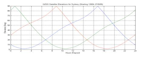
Figure 6. QZSS satellite elevations for Sydney over 24 hours.
