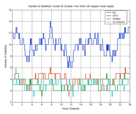
Figure 3. Satellite visibility for Sydney over 24 hours with 40° masking angle (starting 1200h 27 May 2005).
