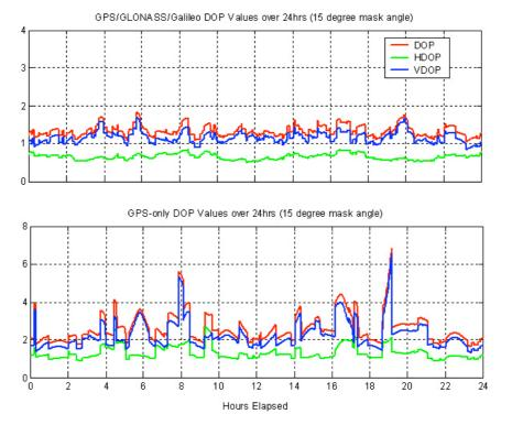
Figure 2. Dilution of Precision values over 24 hours for combined GPS/GLONASS/Galileo (Top) and GPS-only (Bottom) systems with a 15 degree masking angle (starting 1200h 27 May 2005).
