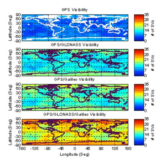
Figure 5. Global snapshot of satellite visibility with 15° masking angle (1200h 27 May 2005).
