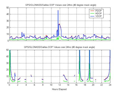
**Figure 4.** Dilution of Precision values over 24 hours for combined GPS/GLONASS/Galileo (Top) and GPS-only (Bottom) systems with a 40° masking angle (starting 1200h 27 May 2005).
