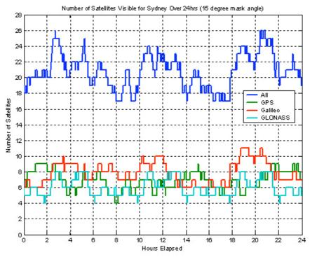
Figure 1. Satellite visibility for Sydney over 24 hours with 15° masking angle (starting 1200h 27 May 2005).
