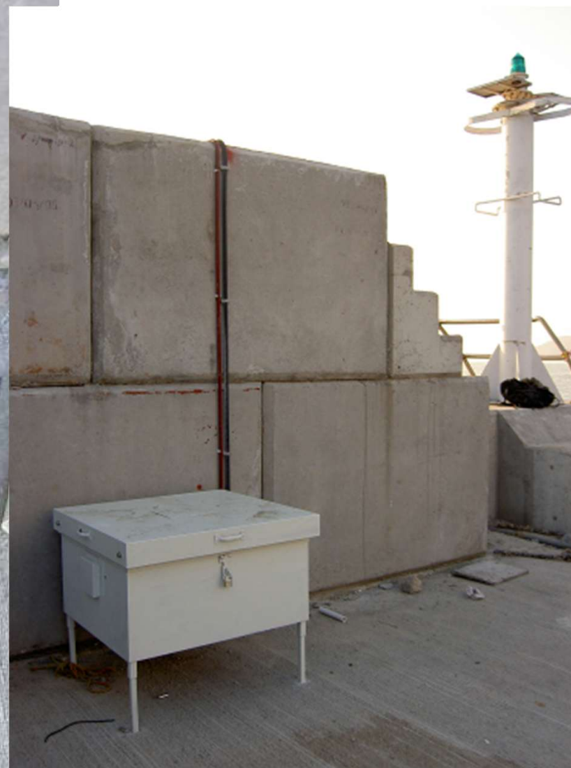
Leica Geosystems GNSS monitoring stations for checking Seawall infrastructure in Hong Kong, PR China
