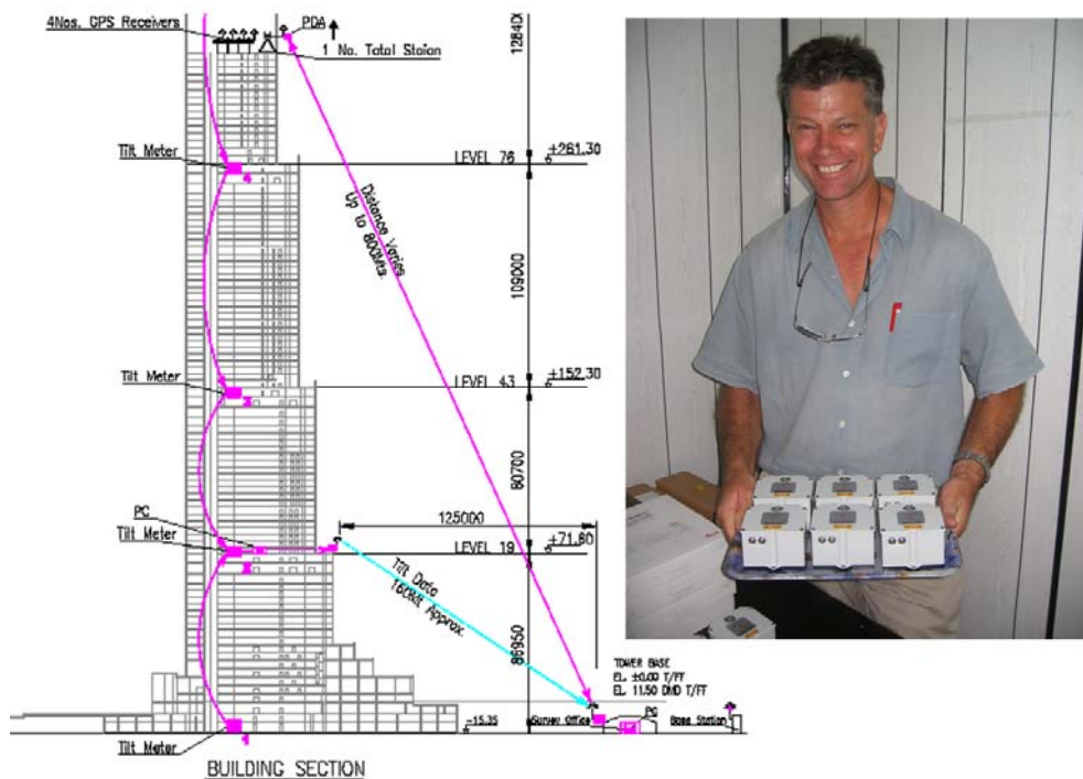
Fig 3: example of designing a Leica NIVEL200 network by Doug Hayes in Dubai.
