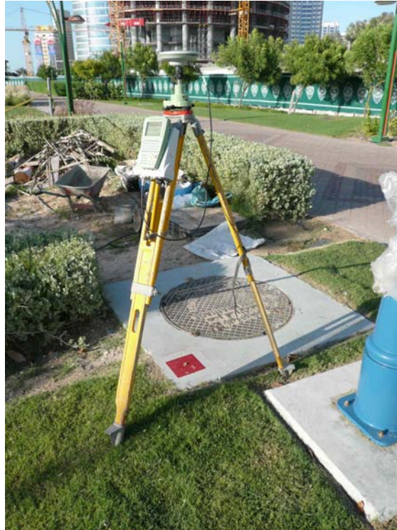
Fig 5: control point re-surveyed by GNSS receiver
