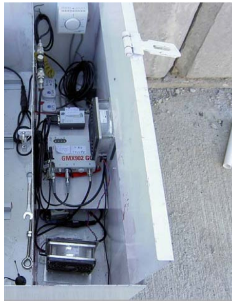
Fig 2: GPS receiver Leica GMX902 with power supply and communication interface
