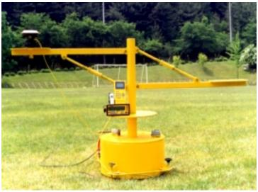
Figure 4. Rotating table used for the RTK-GPS test.
