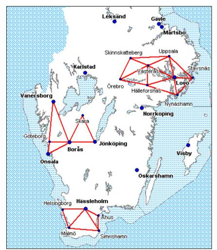
**Figure 7**: The three test platsforms for network-RTK existing at present in Sweden. From top to bottom are the areas for the projects Position Stockholm-Mälaren, New-RTK and SKAN-RTK.
