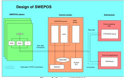
Figure 2: Design of SWEPOS
