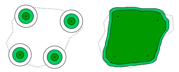
Figure 6: Coverage with single station RTK and network RTK
