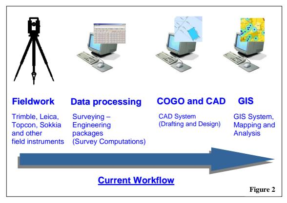
Deficiencies in the above system or workflow is that there are no links between the first step (field measurements) and the final GIS or cartographic map product. This becomes problematic if a new survey is conducted or a new value is determined for some of the contributing survey points to a GIS map layer. This current methodology requires the entire process above be repeated to update GIS or map features.
