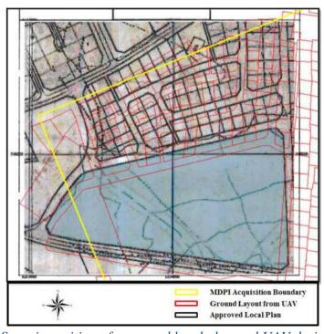
Figure 7: Superimposition of approved local plan and UAV derived line map
