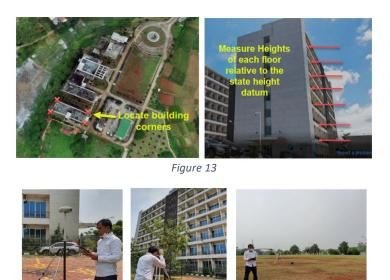
(a) (b) (c) Field Work Image : (a) GNSS CORS, (b) Total Station Reflectorless, (c) UAV Lidar Figure 14
