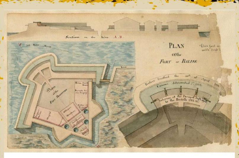
Fig. 6.11. "Plan for the Fort of Balise" with the projected Fort (left) with status report of how far the construction had progressed (right) and side view on top. [Lafon.BaliseFort.1814.HNOC.1970.2.1-
