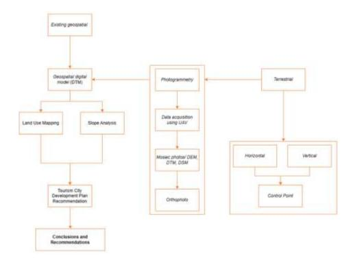
The analysis will be done using an *unmanned aerial vehicle* and a mirrorless camera. This analysis will generate point clouds and orthophotos data. That output will then be used to generate spatial models in the form of terrain models and high-resolution imagery (Caroti et al., 2015; Iheaturu et al., 2022). The specifications of the tools used in this analysis are stated in the table below. The tools are capable to generate 4 cm/pixel imageries and 15 cm/pixel terrain models.
