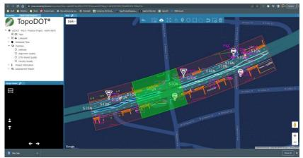
Figure 13: Select tile(s) to download corresponding point cloud data from warehouse
