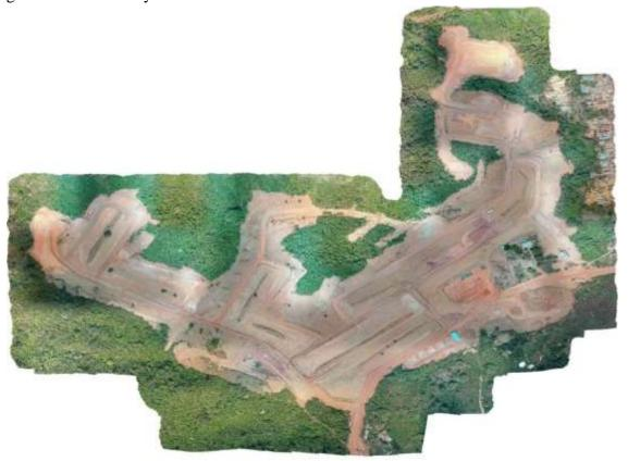
Fig. 6: Digital Elevation Modelling (DEM) generated from Drone Images
