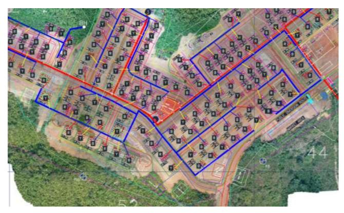
Fig. 22: CAD Design Overlayed on Drone DEM to Check Compatibility
