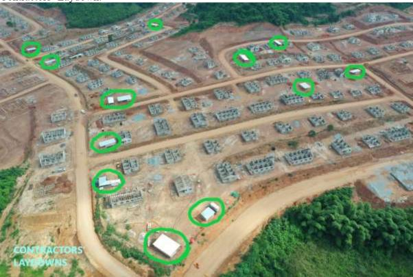
Fig. 11: The designated Contractors' Laydown from the Drone image
