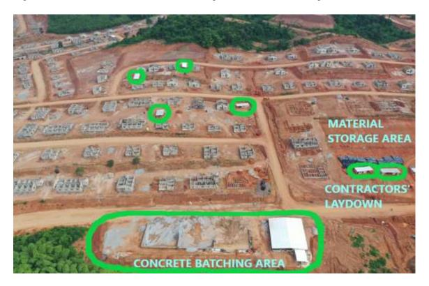
Fig. 10: The Designated areas for Concrete Batching Area, Materials Storage Area and Contractors' Laydown.
