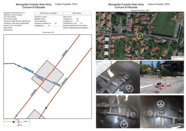
The final map consists of the materialization of the water network containing all the data collected inside, which is delivered to the contracting station with the possibility of being overlaid with any other cartography available to the client, also it has the possibility of updating it in time real through any tablet, or even by the operator himself who performs extraordinary maintenance or new lines.
