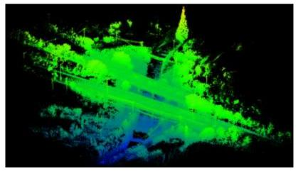
Figure 7 Backpack scanning point cloud data
