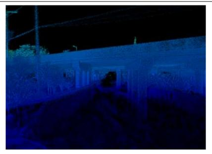
Figure 8 The local point cloud data of bridge pier
