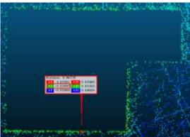
Figure 4 Thickness of wall column measured in CloudCompare
