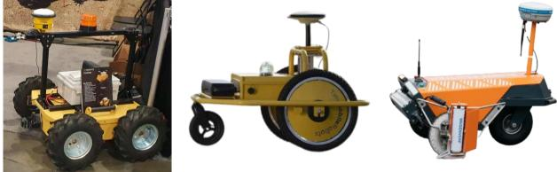
Those robots are perfectly adapted for low accuracy premarking (around 2cm of accuracy) Good for road works and...
