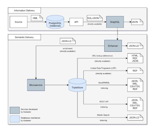
Figure 2 – Architecture supporting the ETL process which produces linked data (Rowland et al., 2022)
