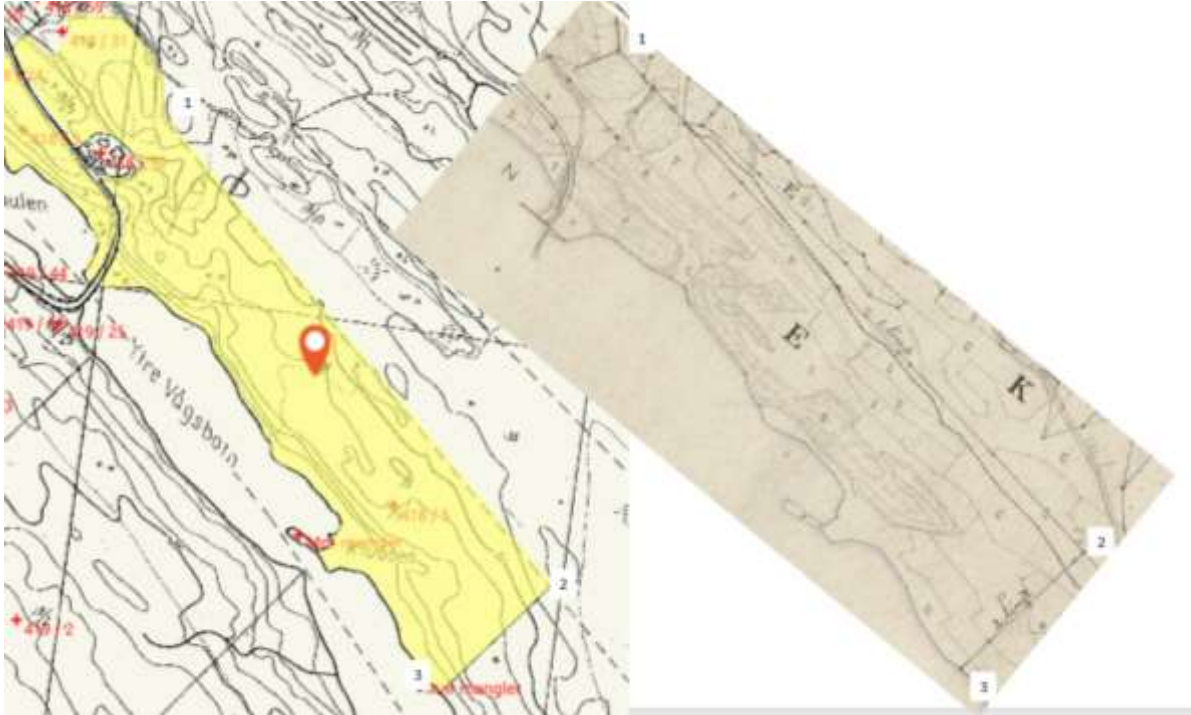
Figure 10. To the left we can see registration in the cadastral map with yellow color and the economic map as background. To the right the land consolidation map. In the land consolidation map the boundary marks set out in the terrain are marked. The boundary line investigated is marked 1-2-3. Source: www.geonorge.no and https://wcarkiv.domstol.no/wcarkiv/kommunelist.wc?ID .
