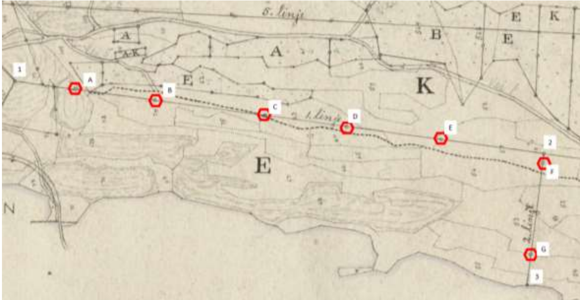
Figure 11. Section of the land consolidation map, showing the investigated boundary line. Points 1 - 3 are corner points, A - G are intermediate markers on the line between the corner points. Source: https://wcarkiv.domstol.no/wcarkiv/kommunelist.wc?ID .
