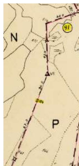
Figure 5. Extract from the LCC-protocol describing the boundary lines and corresponding map-details. Note the description of Boundary no 91, with details about type of marking, point number, (ex No 184), distance from other points and indication of change in bearings/azimuth. Source: https://wcarkiv.domstol.no/wcarkiv/kommunelist.wc?ID
