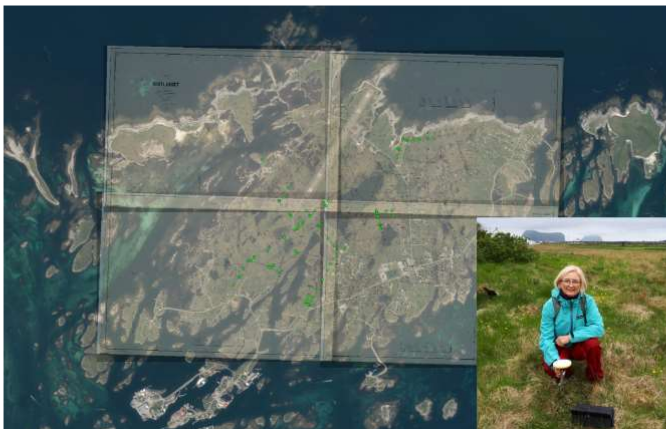
Figure 8. Test of mobile application including cm-GNSS services. Around 100 cadastral monuments were recovered and measured using Qfield-application. Even personnel not trained as a surveyor could perform registration without major
