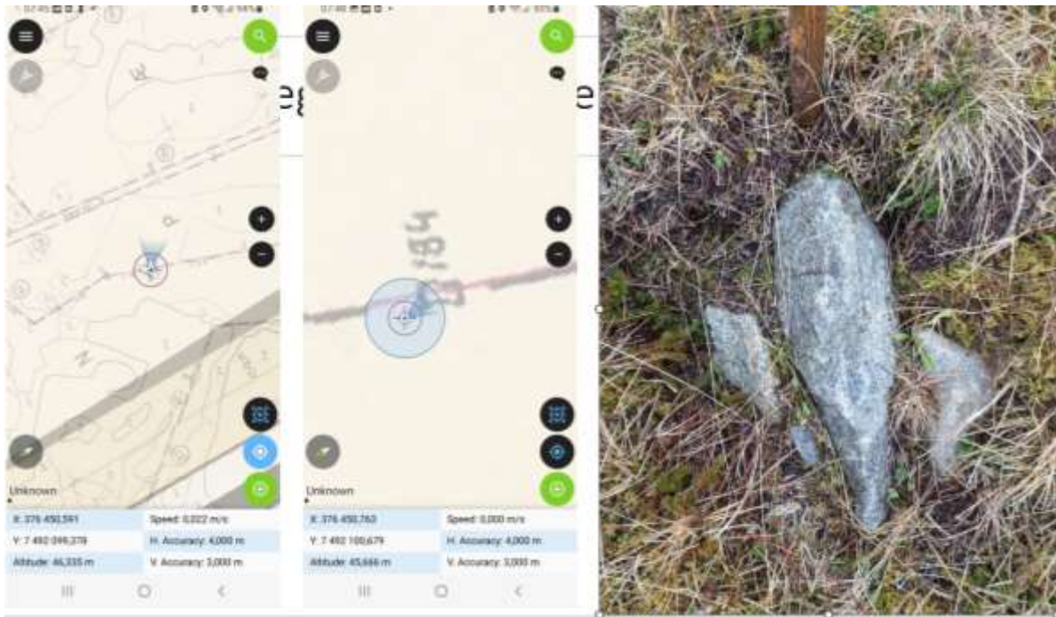
Figure 6. Using the application Qfield on a mobile platform – we were able to find old boundary stones/markers in the Klakk area. Within a circle of 4 meters radius from the detail in the map/application, we were able to find most of the cadastral monuments in the area. Source: Screenshot Qfield and https://wcarkiv.domstol.no/wcarkiv/kommunelist.wc?ID . Photo: Per Ove Røkke.
