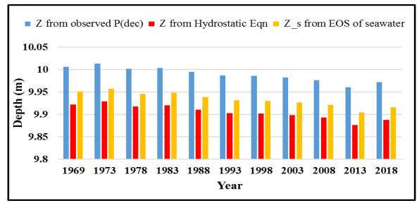
Figure 3: Temporal trend of Derived Depth from hydrostatic equation, Equation of state (EOS) and the theory of equivalence of observed pressure to depth to depth from 1969 to 2018.
