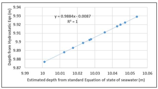
Figure 4: Linear trend between the depth from hydrostatic equation and EOS
