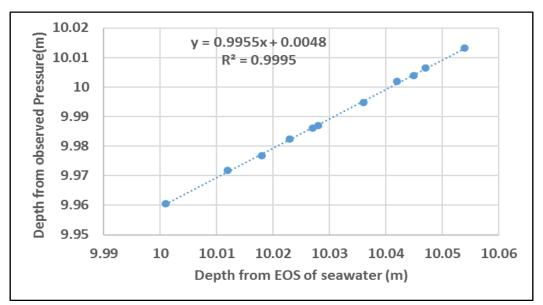
Figure 4: Linear trend between the depth from observed pressure and EOS
