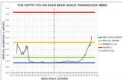
*Figure 11. Depth TVU Graph for each beam angle of MBES Transducer* Based on the graphical image, the width of the MBES swath between -70 to 68 degrees could reach the depth of TVU in order 1a/1b in case the survey area is relatively flat.
