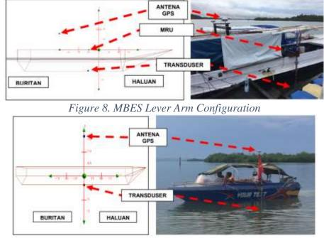
Figure 9. SBES Lever Arm Configuration
