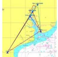
Figure 7. Baseline Configuration for GNSS Observation
