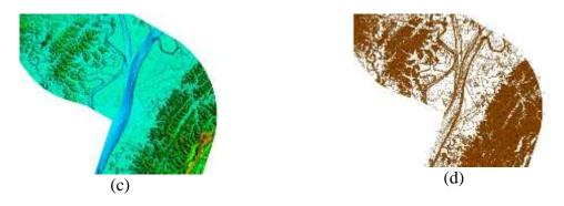
Figure 15. (15a) Ground LiDAR with elevation reference are refer to Benchmark HK.64.09.046, (15b) Bathymetric Data in River Area (Point), (15c) Digital Terrain Model from combination of Ground LiDAR and Bathymetry, (15d) Contour Data derived from DTM in fig. 15c.
