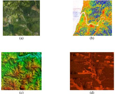
Figure 14. (10a) Aerial Imagery from Airborne LiDAR, (10b) 3D Point Cloud already classified, (10c) Digital Terrain Model (DTM), (10d) Digital Surface Model (DSM)
