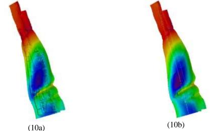
Figure 10a and 10b. (10a) Seafloor DTM before Patchtest Callibration (10b) Seafloor DTM after Patchtest Callibration
