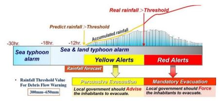
Figure 2. The flow chart of rainfall-based Debris Flow Warning Model
