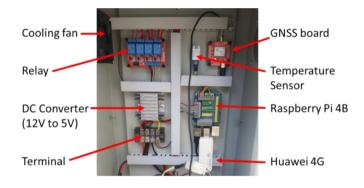
Figure 5 The example of electronic equipment in a waterproof sheet steel wall box.
