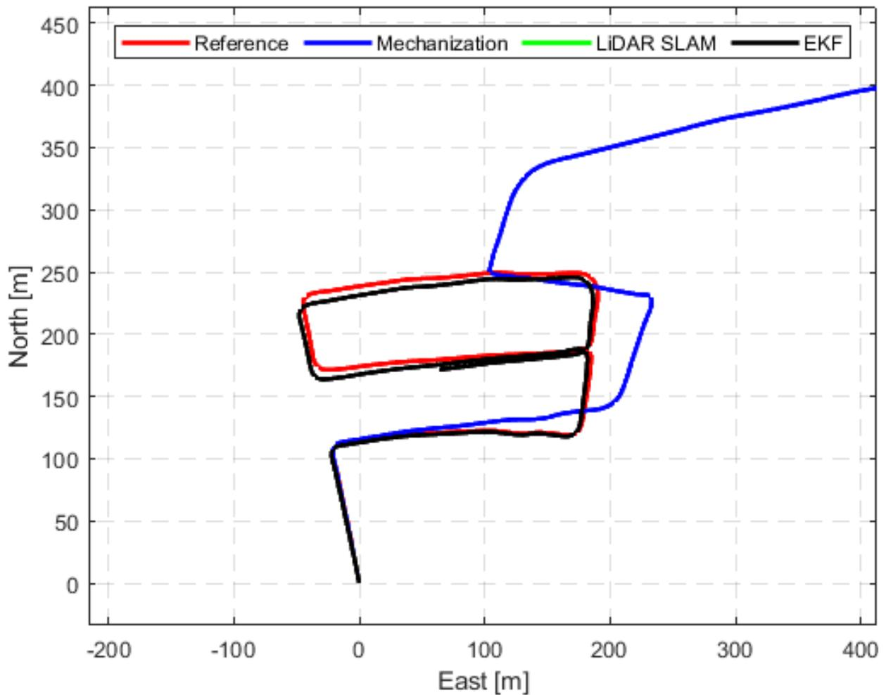
Figure (3): Residential dataset – complete GNSS signal outage: comparison of trajectories
