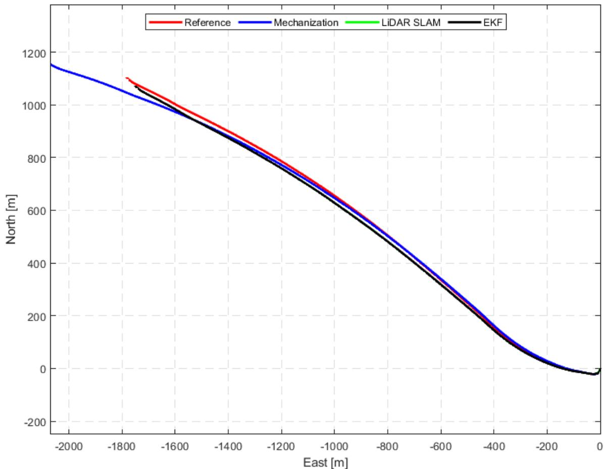
Figure (5): Highway dataset – complete GNSS signal outage: comparison of trajectories
