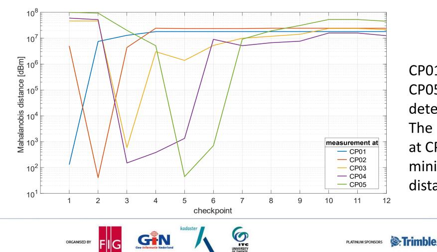
CP01, CP02, CP03 and CP05 have been correctly determined The on-line measurement at CP04, however, has its minimum Mahalanobis distance at CP03
