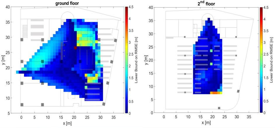
Low CRLB values (dark blue) indicate higher positioning accuracies during the on-line phase, while higher values (red) mean lower accuracy
