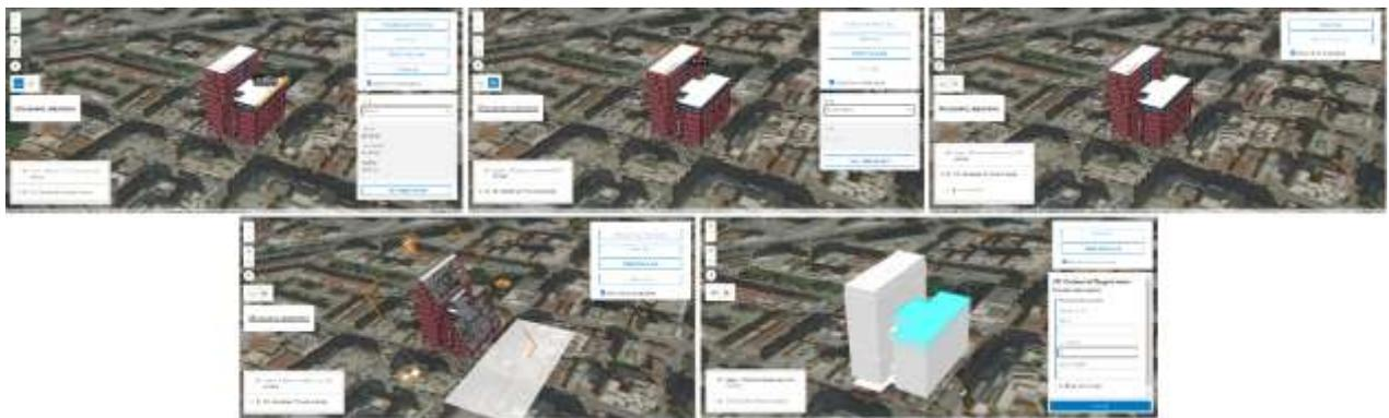
Figure 3: Top-row (left to right): the 3D length measurement tool; the 3D area & perimeter measurement tool; and, the layer management tool. Bottom-row (left to right): the building slicing tool; and, the editor tool.
