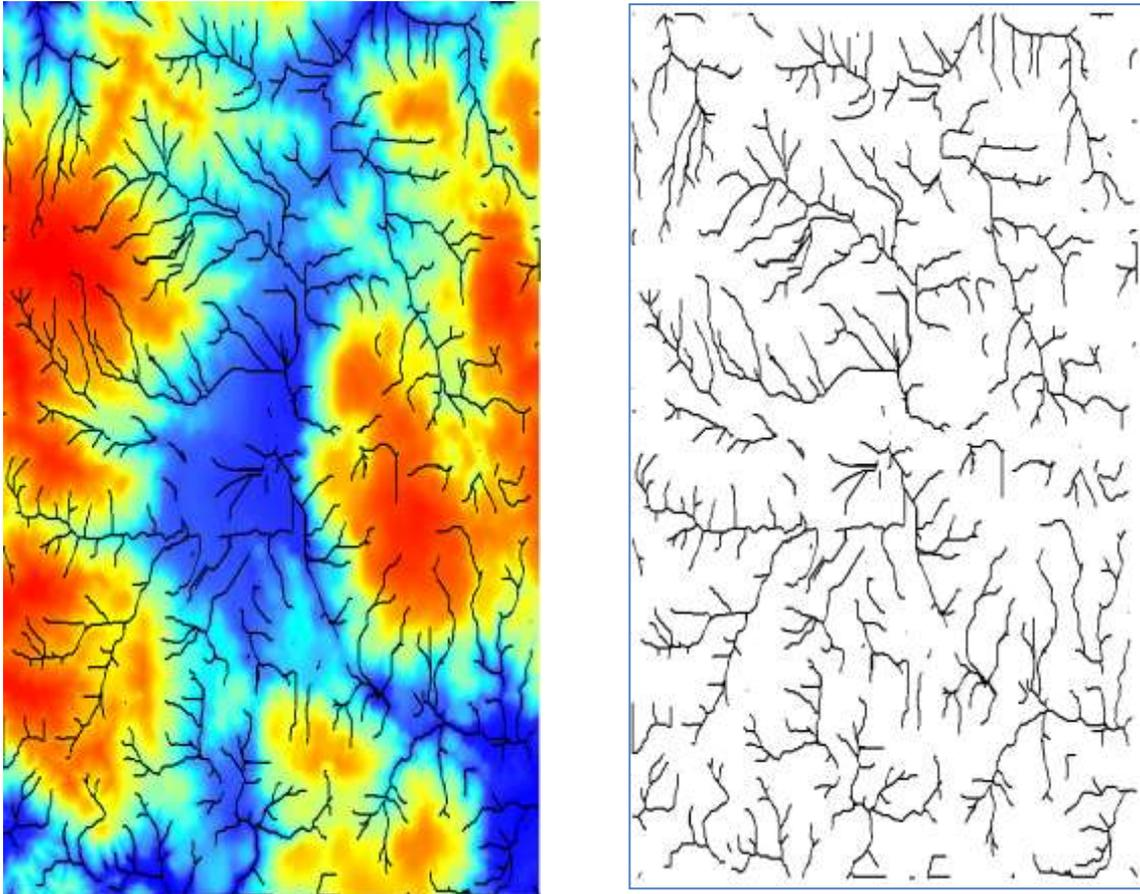
*Figure 6. Digital terrain model and derived riverbeds with a flow accumulation parameter of 800 cells and their result.*
