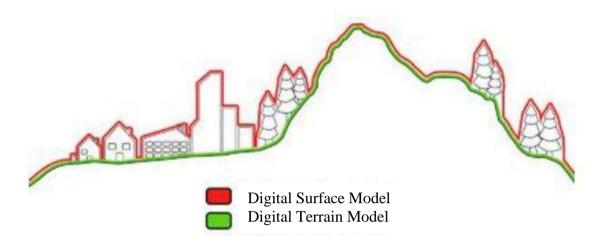
Using the Digital Terrain Model and Digital Surface Model, calculations are made for the difference between the two. This provides a representative feature height that is used in capture interpretation. When the height tool is activated the cursor provides the hight in metres (m) as the cursor is moved over features, the number adjusts dynamically to display the correct figure.
