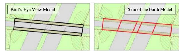
Elevated features not part of the skin of the earth such as a road or pavement on a bridge, will be captured with level information and obscured detail will be integrated into the ground level data. Data at the ground level can utilize the DTM and elevated features will be mapped to the DSM to enhance and generate 3D data in downstream systems.
