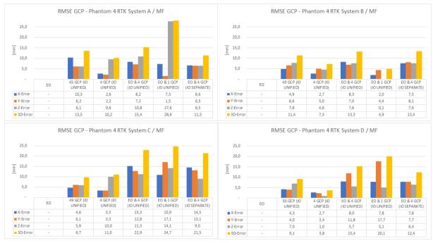
Fig. 6: RMSE values at the control points (CP) depending on the type of orientation (direct: ÄORI – indirect: GCP – integrated: ÄORI+GCP) (systems A - D)
