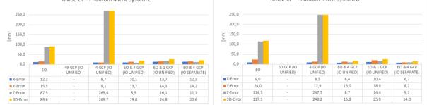
Fig. 7: RMSE values at the control points (CP) as a function of the orientation type (direct: EO - indirect: GCP - integrated: EO+GCP) (systems A - D).
