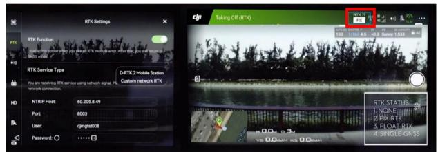
Fig. 2: Definition of RTK parameters using the GS PRO App (Image: Manufacturer)
