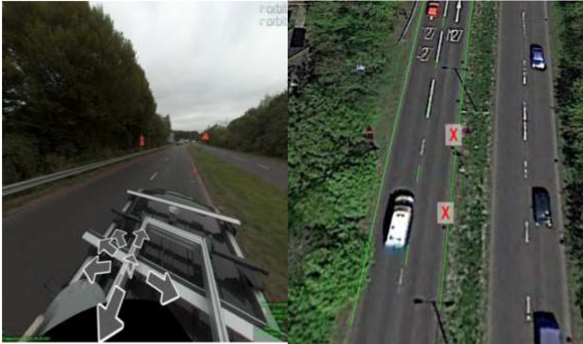
Figure 5. Extraction of road infrastructure elements (left), obtained .kml file in Google Earth (right)
