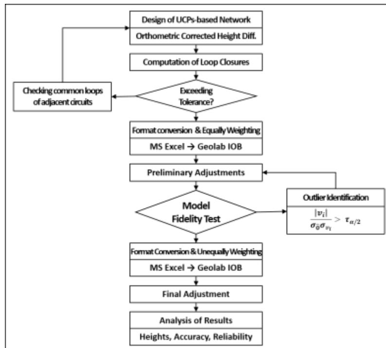
Figure 7. A procedure of UCPs-based levelling network adjustments.
