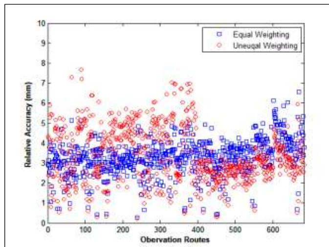
Figure 10. Relative accuracy of the levelling routes.
