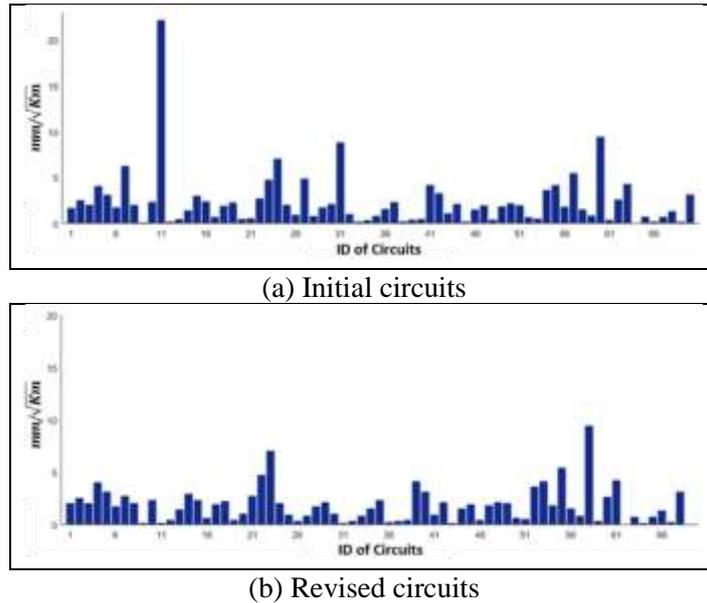
Figure 9. Standardised misclosures of the circuit loop closures.
