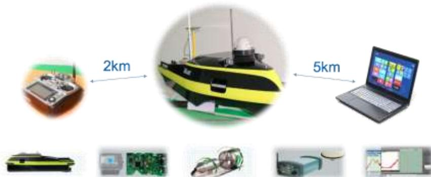
This advanced and autonomous system consists of the vessel body, excellent echo sounding module and positioning module, of course, the data communication system and the controlling system are included.
