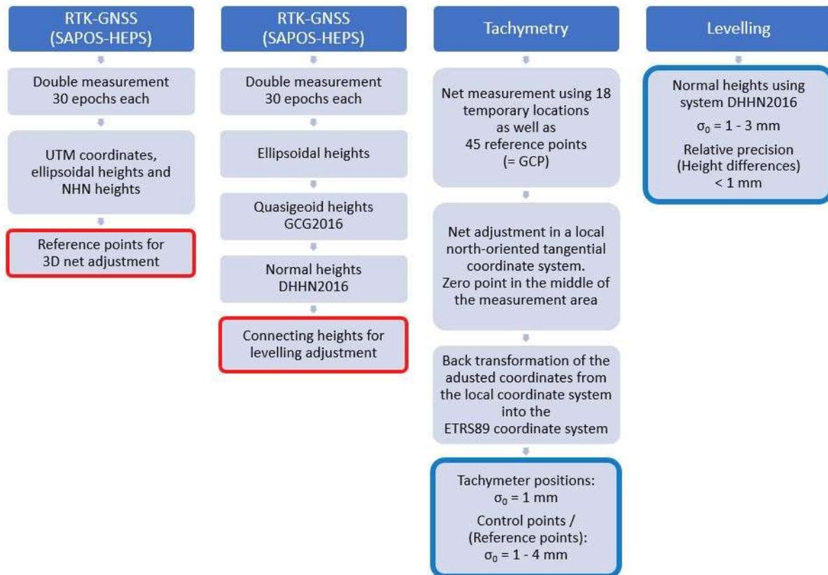
Fig. 3: Workflow of geodetic measurements and data processing (GCG2016 - German Combined QuasiGeoid, the height reference for the transition between geometric heights in ETRS89/DREF91 and physical heights in DHHN2016, the German height reference system).
