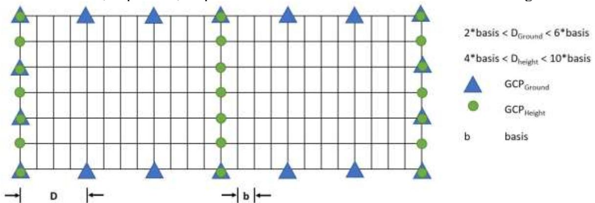
Fig. 6: Schematic arrangement of GCPs during (analogue) image flight (Kraus 1994)
