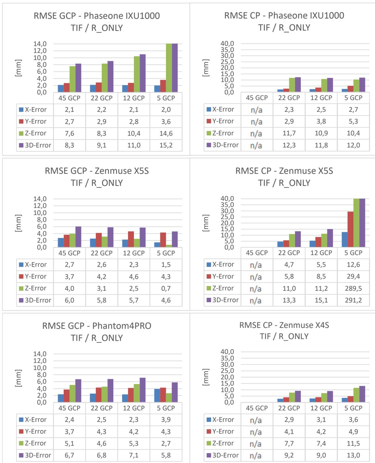
Fig 9: RMSE values at GCPs (left) and CPs (right). Flight arrangement: R. Calculation: Agisoft PhotoScan. Note scaling.
