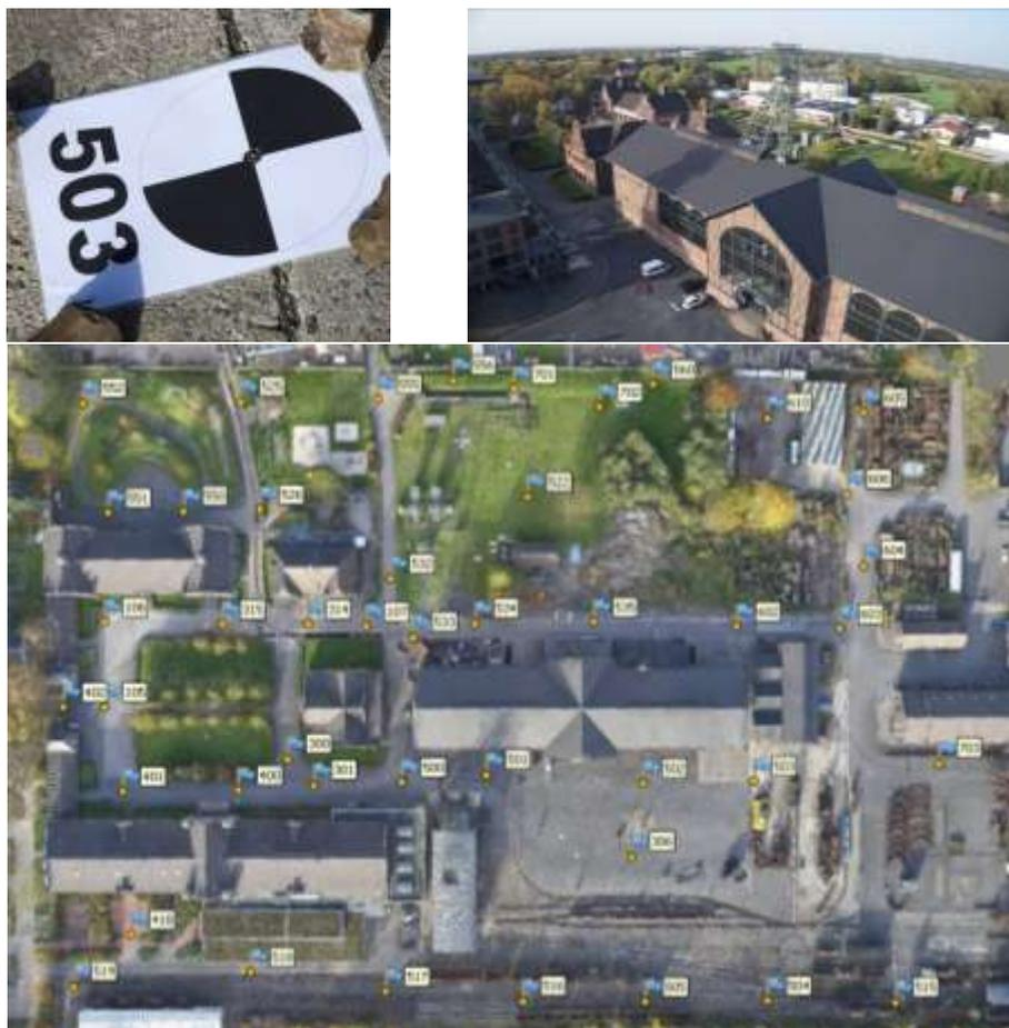
Fig. 2: UAV test field Zollern colliery. Top: Target for signaling the GCPs and view of the area. Bottom: Point cloud with signalized GCPs (UAV flight from October 2017)
