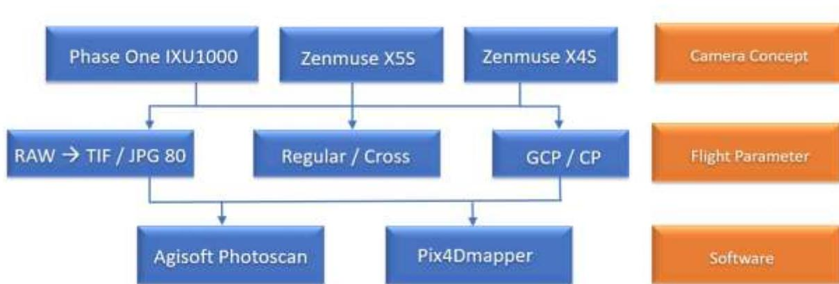
Fig. 5: Parameters influencing the geometric quality of the image blocks
