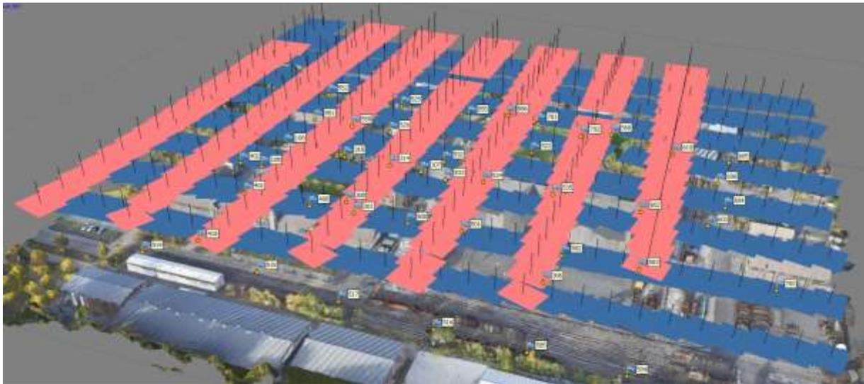
Fig. 4: Flight arrangement Regular (R) and Cross (C), (Image block with Zenmuse X4S)
