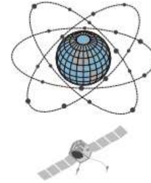
Galileo 3 Orbital planes 27 Satellites + 3 spares 56° Inclination angle Altitude 23,222 km
