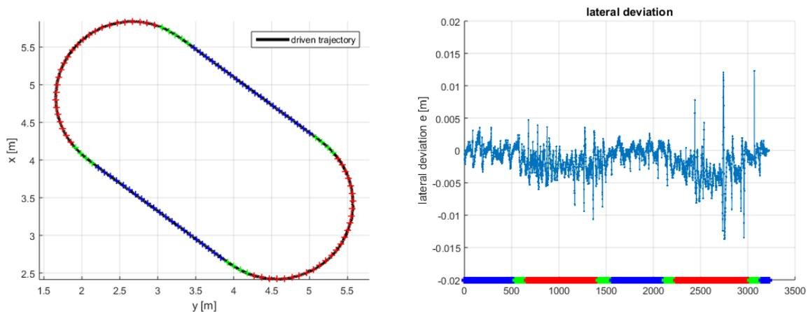
**Figure 6: Oval trajectory (left), lateral deviations (right)**
