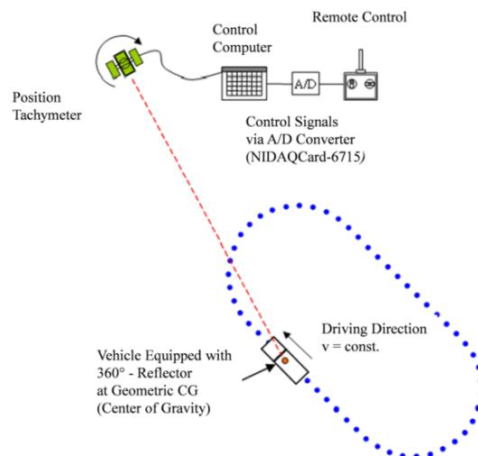
**Figure 5: Experimental setup for evaluation (Beetz 2012)**
