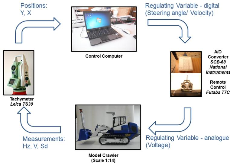
**Figure 1: Hardware components of the simulator**
