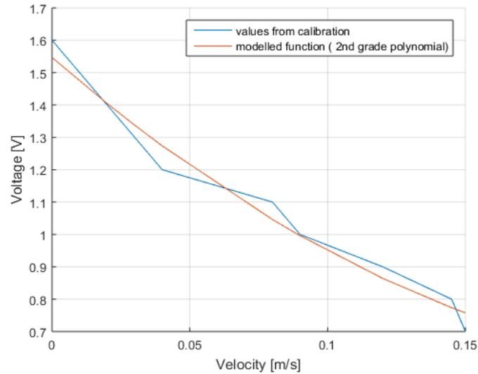
**Figure 4: Transfer function between voltage and velocity**
