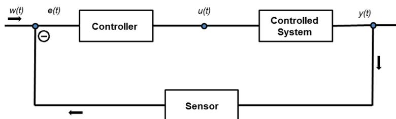
**Figure 2: Closed-loop-system**
