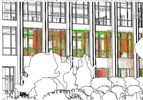
Fig. 4 As-built survey with point cloud and BIM model
