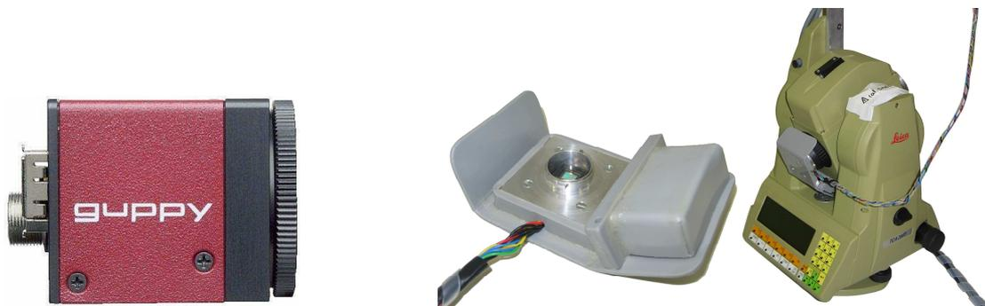
Figure 2. (Left) Guppy CCD camera as available on the market. (Right) Transformed CCD camera. The left picture shows the CCD sensor and the mechanical interface for Leica instruments. The right picture shows the camera mounted at the telescope of a TCA 1800. This adapted flat layout allows to measure even in zenith direction
