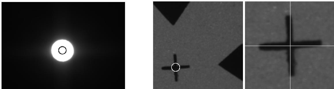
Figure 3. (Left) Example of a lamp measured by QDaedalus with center of mass. (Right) Example of a point measured by QDaedalus with template least square matching algorithm.
