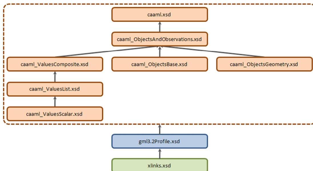
Figure 2 Schema file structure of CAAML version 5.0
