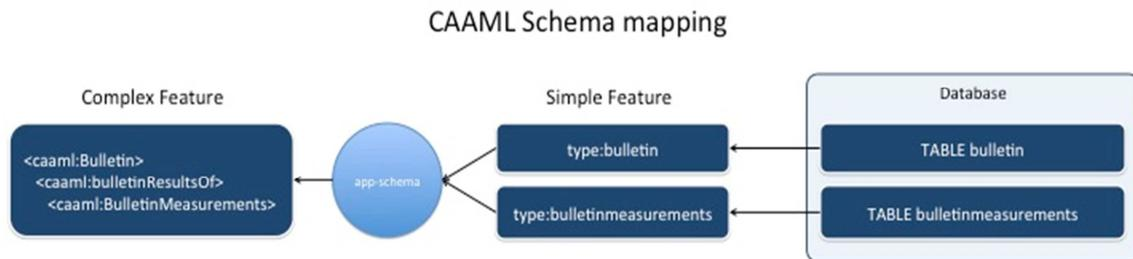
Figure 4 Simple feature mapping of the CAAML complex feature
