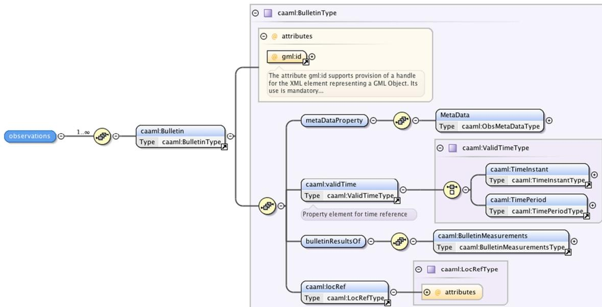
Figure 3 XML schema definition for CAAML bulletin type asserted in the EAWS profile
