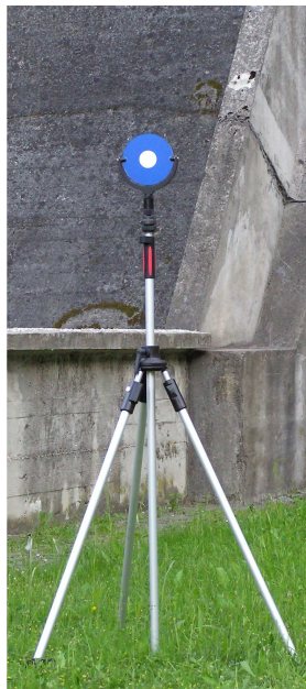
Fig 7. View of Leica's target which guarantee high precision of determining its center on the scan.
