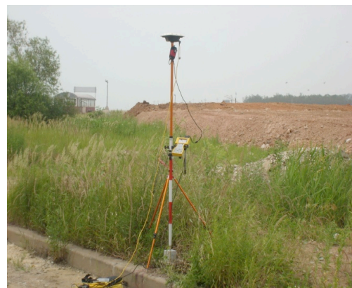
<Figure 3> Installation of RTK
